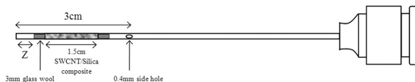
Fig. 1. Schematic of needle trap device with side hole, glass wool and SWCNTs/silica composite as sorbent.
